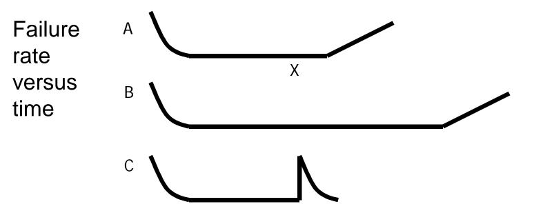
Rebuilding equipment in Figure A at Point X may result in Figure C instead of Figure B
